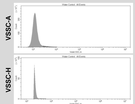
HPLC water was used as a control for instrument cleanliness and particulate contamination. As can be seen above, the instrument was clean and there was minimal background.
