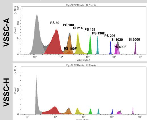
The CytoFLEX Sizing Beads are composed of a mixture of latex and silica NIST-traceable size standards, as well as fluorescent microparticles. They are evenly distributed and spread across the complete VSSC dynamic range for the CytoFLEX.
