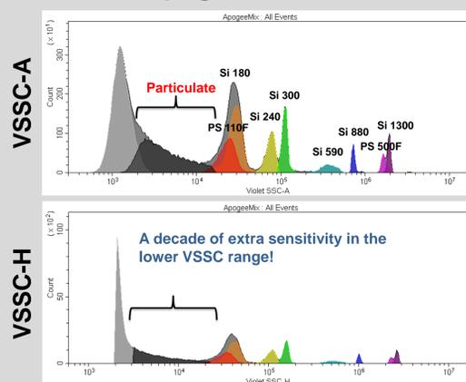
The ApogeeMix Beads are also composed of a mixture of latex and silica beads, including several fluorescent microparticles. These beads contain a significant amount of particulate in the lower size range, they are very unevenly distributed, and have a limited dynamic range.
